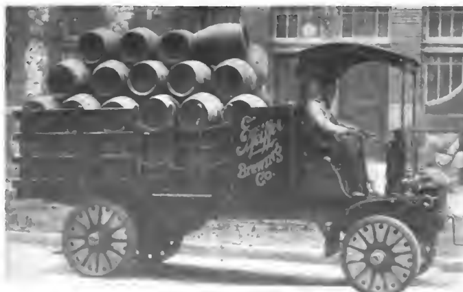
Fig. 2—Three-ton power wagon in brewery service, with open cab, steel wheels, dual rear tires, and a full load
